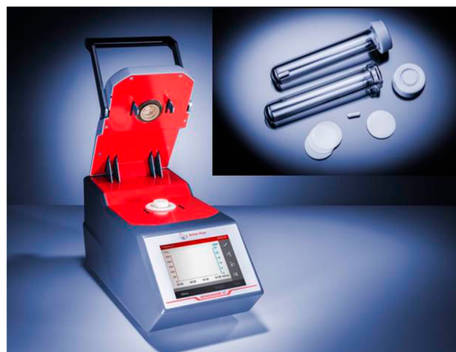
Figure 2. Monowave 50 reactor (Anton Paar GmbH) with open cover and 10 mL glass vials with silicone cap, septa, and stirring bar. Image copyright Anton Paar GmbH (ref 11).
